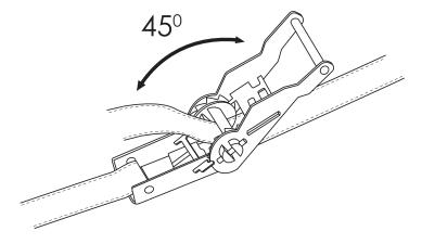
4b. Crank the handle to tighten the strap until it feels taut and secure.
