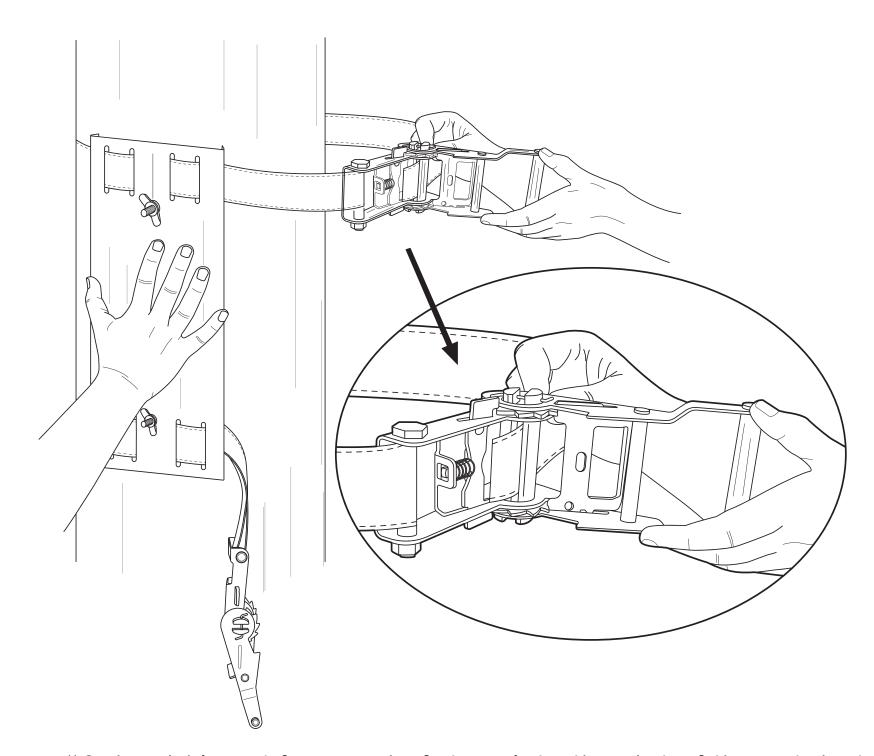
Person #2 should insert free end of strap into the slot of the ratchet buckle.
